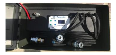
14. Disconnect the cigarette lighter adaptor and roll up the cable secure with the Velcro and store it in the CO2 Ammo air box.
