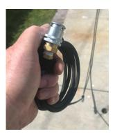
13. Roll the hose up until you reach the CO2 Ammo air box. Wrap the Velcro around all the loops. Repeat with the other pair of hoses. Place the hoses in the box.
