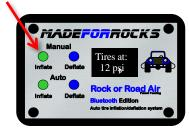
**Note:** Pressure display is not accurate during manual inflation.
